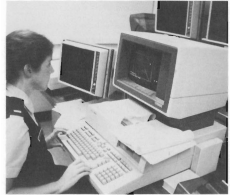
Before flight, every move of the great arm is simulated at the Johnson Space Center using HP equipment. Here Air Force 1st Lt. Gail Ramsey enters data on an HP 9000 attached to plotter and graphics translator with three cathode ray displays. She sees the arm's motion from three viewpoints.
