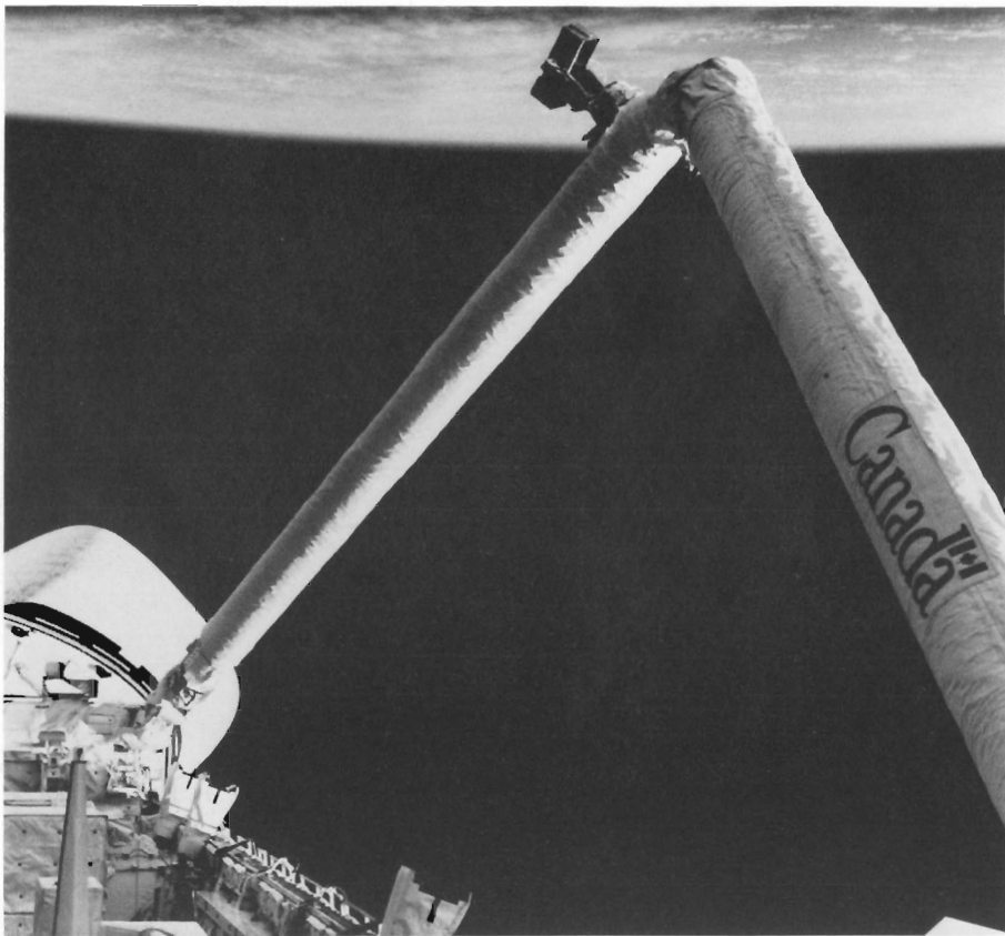
During flight, the remote manipulator system's arm reaches over to grab a payload (left) for deployment into space. View is from cabin's aft window, looking into wide-open bay.
